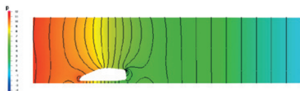
Figure 5. Car in a wind tunnel: simulated pressure (Stokes flow)
