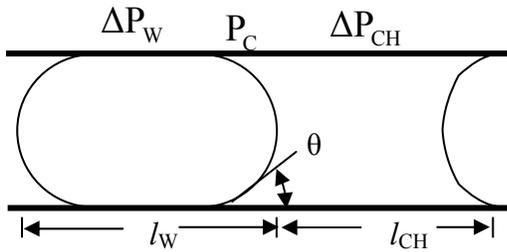
Figure 2: Pressure drop along single slug unit.
