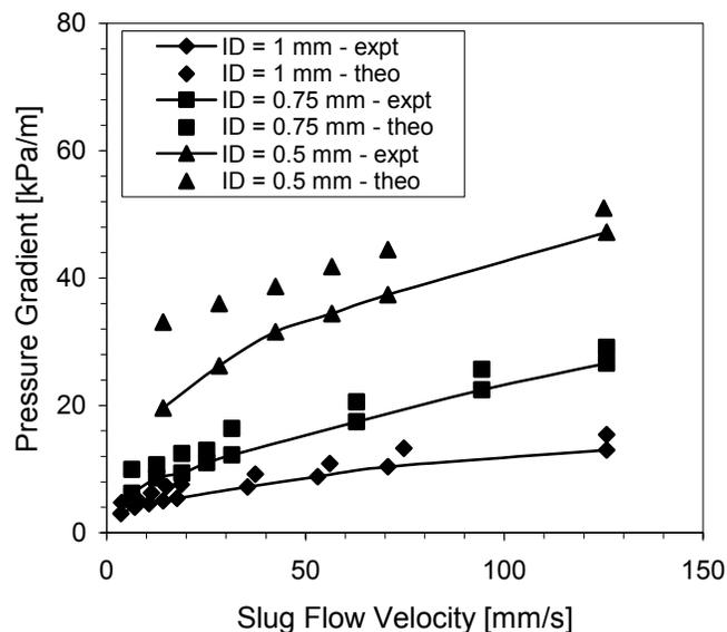
Figure 6: Pressure drop in the capillary millireactor for different capillary internal diameters.
