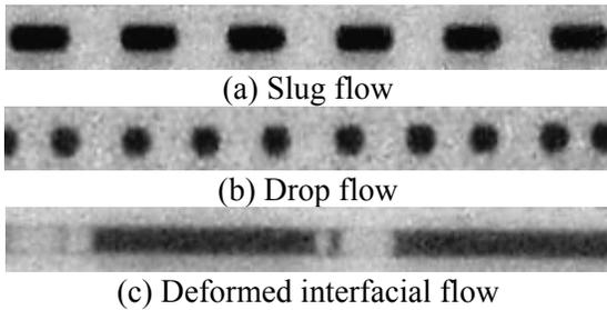
Figure 3: Flow structures in alternating liquid-liquid flow regimes in capillary microreactor (Y-junction ID = 0.5 mm, Capillary ID = 0.5 mm)
