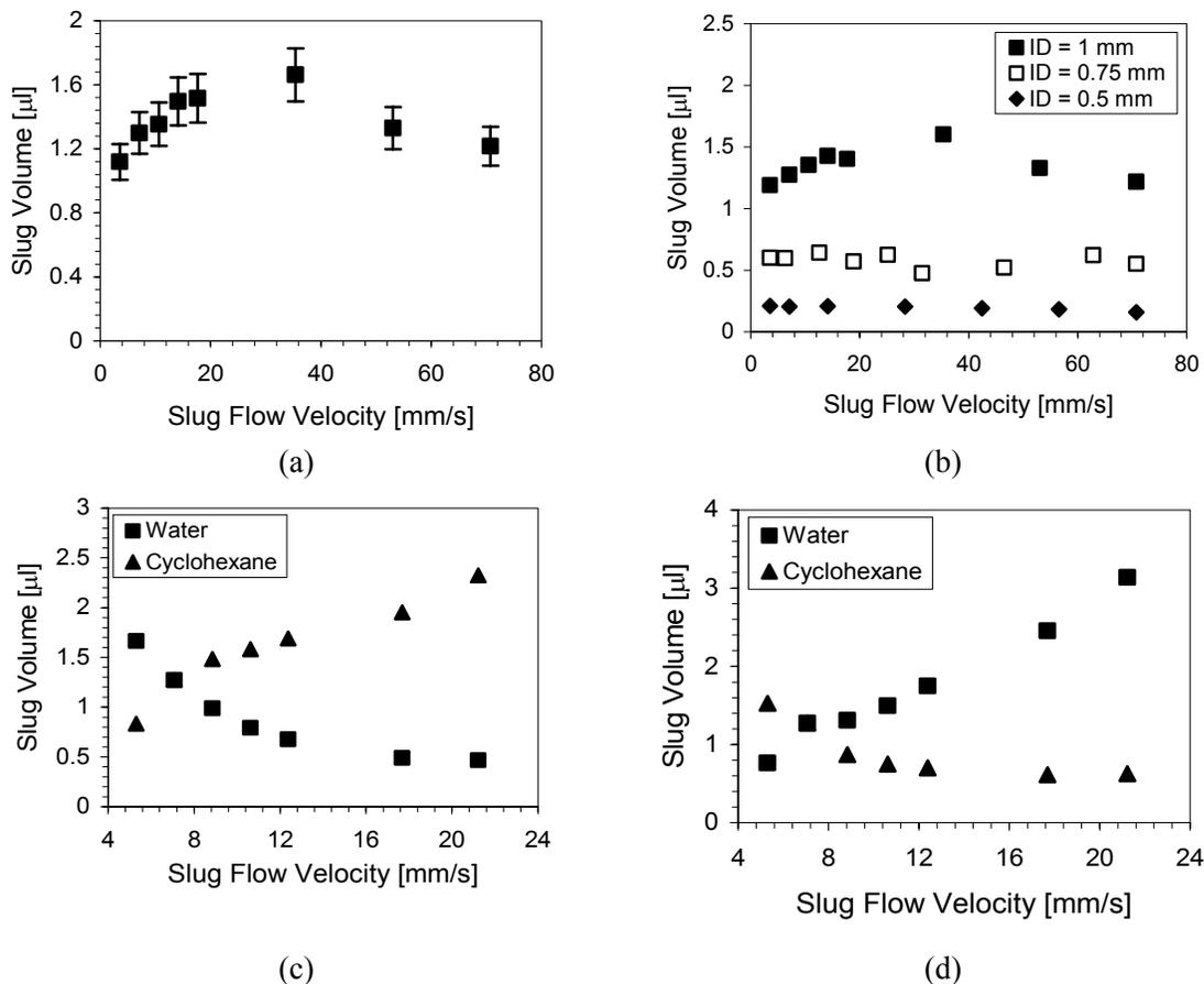
Figure 5: Slug volume as a function of slug flow velocity. (a) Variation in slug size (capillary ID = 1 mm), (b) Effect of capillary diameter on slug volume, (c) Slug volume at constant flow rate of water, 10 ml/hr, and (d) Slug volume at constant flow rate of cyclohexane, 10 ml/hr.
