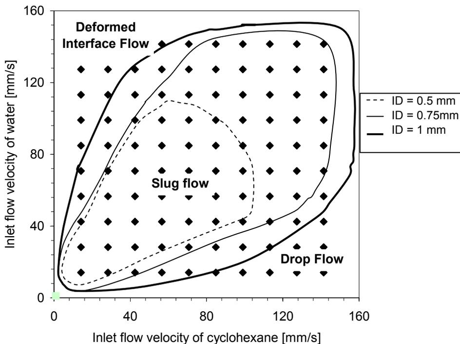
Figure 4: Observed flow regimes for various capillary diameters with different inlet velocities in the Y-junction mixing element.
