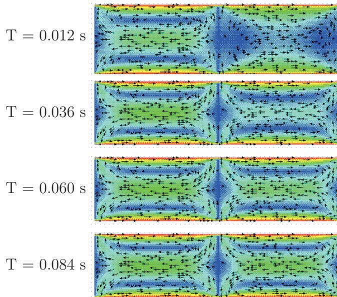
Fig. 3. Flow development for different viscosities in a slug unit (Left slug kinematic viscosity =  $0.3 \times 10^{-5} m^2/s$  and right slug kinematic viscosity =  $0.3 \times 10^{-3} m^2/s$ )
