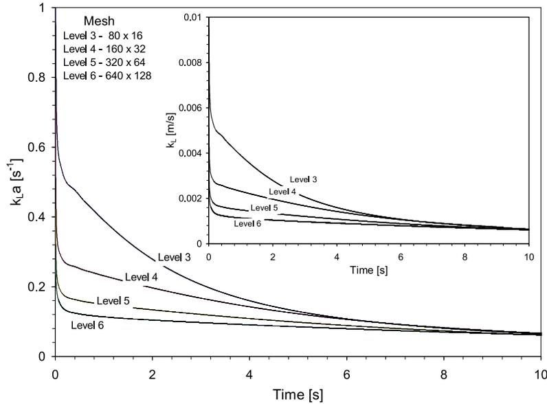
Fig. 5. Volumetric mass transfer coefficient,  $k_{La}$  and mass transfer coefficient,  $k_L$  for different level of refinement
