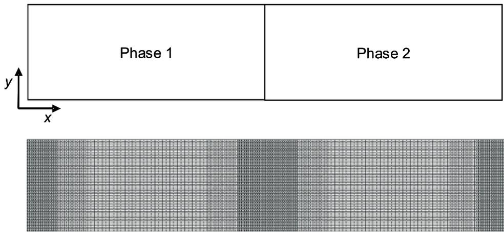
Fig. 2. Computational domain and mesh, showing the more refined mesh in the vicinity of the interface and periodically connected interface
