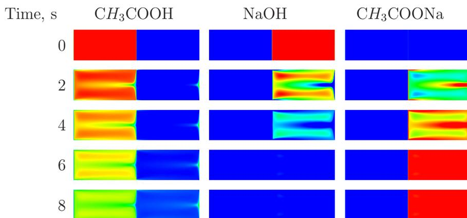
Fig. 9. Snapshots of concentration profiles of CH<sub>3</sub>COOH, NaOH and CH<sub>3</sub>COONa(slug length = 1.9 mm, slug flow velocity = 3.33 mm/s)
