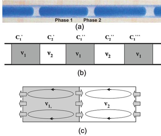
Fig. 1. Liquid-liquid slug flow (a) Experimental snapshot, (b) Schematic representation of the slug flow, and (c) computational domain
