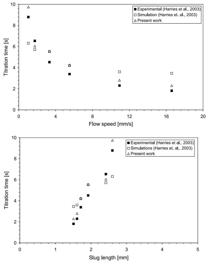
Fig. 10. Plot of titration time vs flow speed and titration time vs slug length
