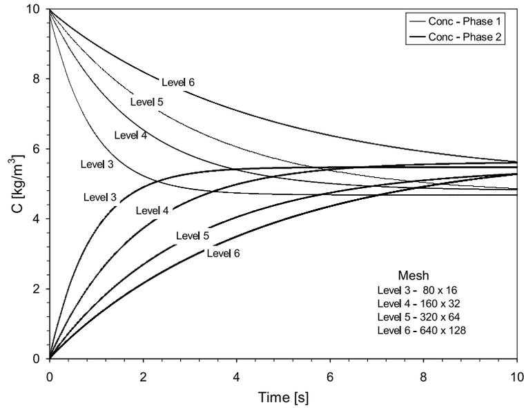
Fig. 4. Concentration profiles for different level of refinement
