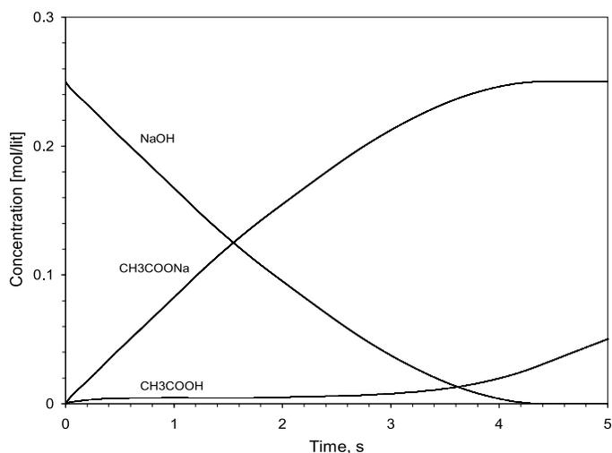
Fig. 8. A typical plot of average concentrations of three species in water slug (slug length = 1.7 mm, slug flow velocity = 5.5 mm/s)
