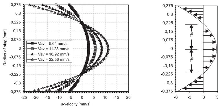
Fig. 4. Parabolic velocity profile inside the slug (aqueous slug, length = 2.379 mm and diameter = 0.75 mm)
