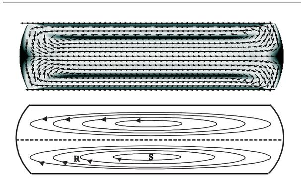
Fig. 3. CFD simulated velocity vectors and schematics of velocity patterns showing recirculation zone (R) and stagnant zone (s)
