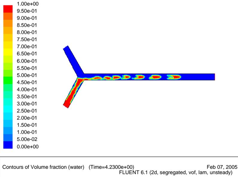
Fig. 6. Flow simulation without wall adhesion in a microreactor of 1 mm diameter for oil-water system. ( $u_1=10$  mm/s and  $u_2= 10$  mm/s)
