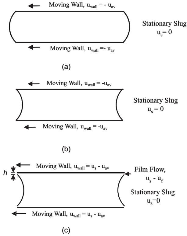
Fig. 2. Computational domains and boundary conditions for single-phase simulations ( $u_{wall}$  is wall velocity): (a) Aqueous slug without and with film, (b) Organic slug without film and (c) Organic slug with film
