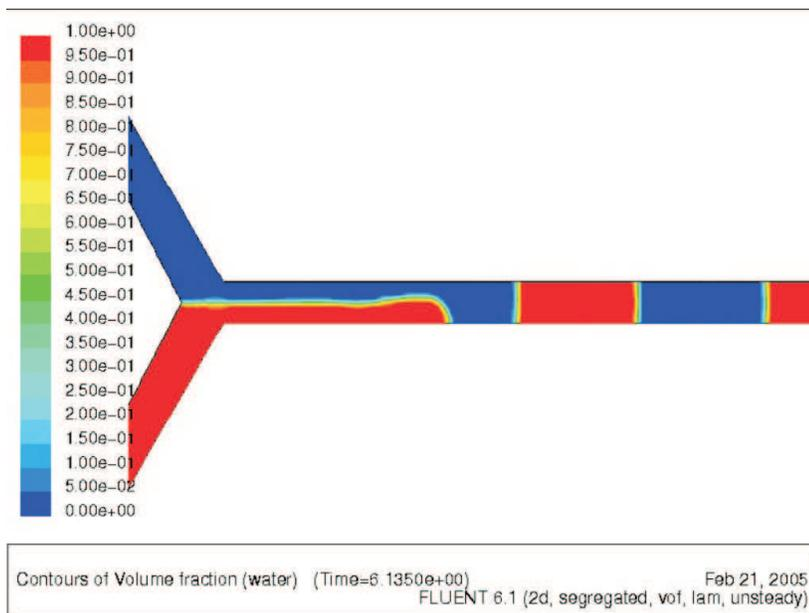
Fig. 7. Slug flow formation at Y-junction in a capillary microreactor of 1 mm diameter for oil-water system. ( $u_1=10$  mm/s,  $u_2= 10$  mm/s,  $\theta_w=90^0$ )
