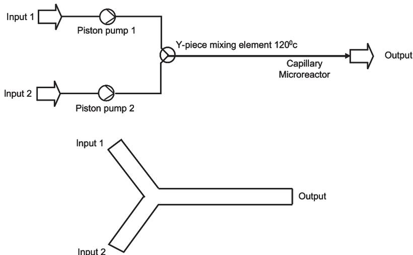
Fig. 5. Schematics of experimental set up and computational domain
