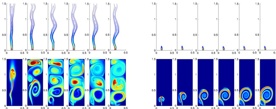
Figure 3: Physical absorption (left) and reaction-enhanced absorption of  $\text{CO}_2$  (right) represented by gas holdup distribution (top) and dissolved  $\text{CO}_2$  concentration (bottom).
