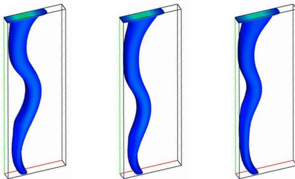
Figure 2: Gas holdup distribution for the locally aerated flat bubble column.
