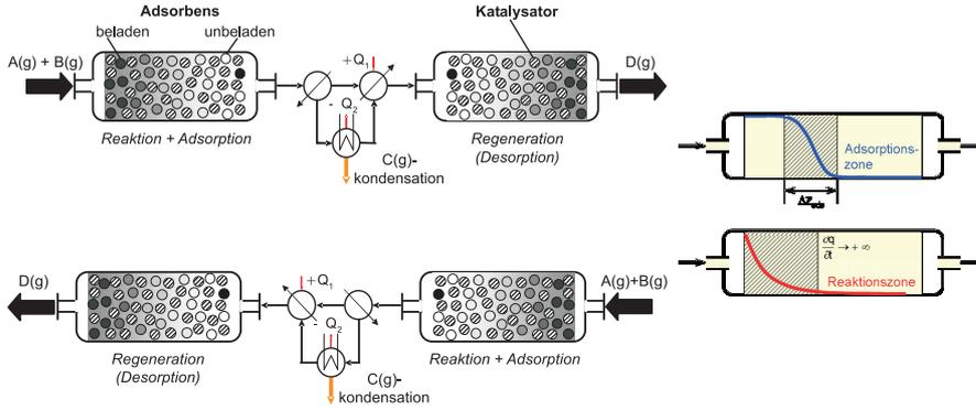
Figure 2: Adsorptive reactor with production- and regeneration-cycle (left) and typical shifted fronts (right) within the cycle.
