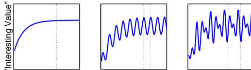
Figure 4: Principle transient behaviour of a stationary, (cyclic) instationary and chaotic processes (left to right)
