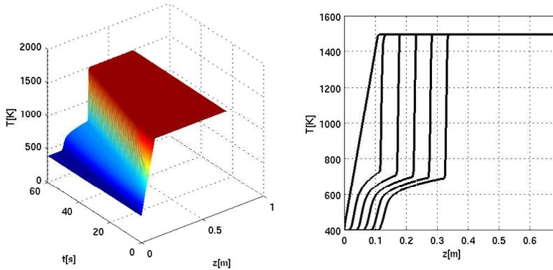
Figure 8: Thermodynamically determined endothermic reaction forms shocks
