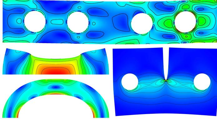
Figure 2: Displacements and von Mises stresses for four prototype configurations (STEELFRAME, BLOCK, PIPE and CRACK), computed with the GPU-accelerated solid mechanics application FEASTsOLID.
