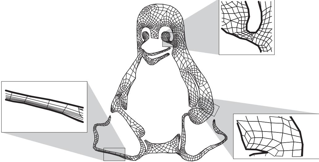
Figure 1: Exemplary Tux geometry. Important features of FEAST’s discretisation approach are highlighted: Globally unstructured, locally structured grids; anisotropic refinement and regular refinement to generalised tensorproduct grids.
