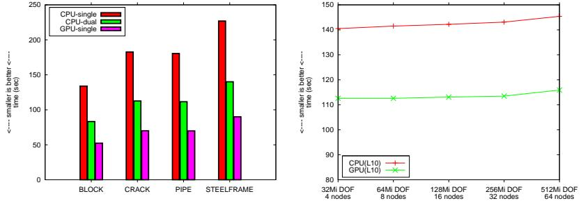
Figure 3: Timings for a singlecore, a dualcore and a GPU solver (left), weak scalability results (right). All computations were performed with the GPU-accelerated solid mechanics application FEASTSOLID.
