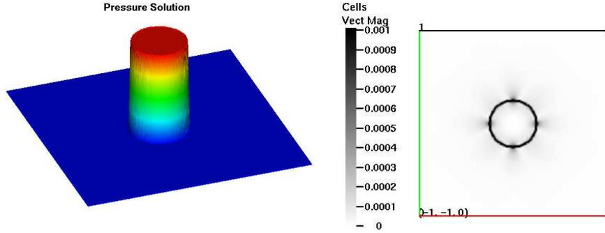
Fig. 2. Pressure and resulting spurious velocity for the 'static bubble' configuration
