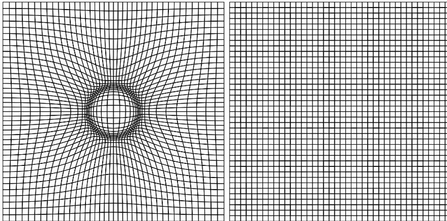
**Fig. 6.** Adapted vs. ‘simple’ mesh (both  $NEL = 1,600$ ) on mesh level 4
