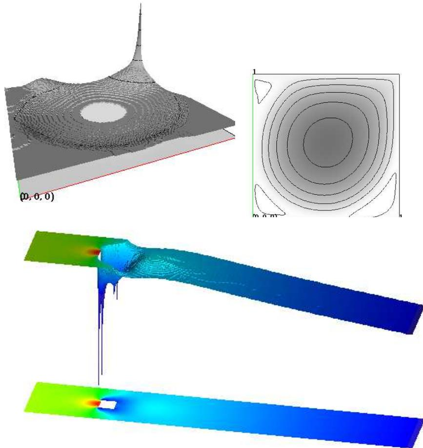
**Fig. 1.** Singularity of the pressure for the ‘Driven Cavity’ configuration, together with the streamfunction, and for ‘flow around a square’
