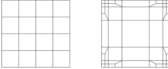
**Fig. 3.** Two different coarse meshes for ‘Driven Cavity’
