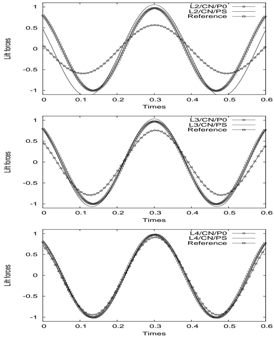
**Fig. 5.** Lift coefficient for various mesh levels ('L=2-4') for Crank-Nicolson 'CN' as time-stepping scheme with pressure separation 'PS' and without pressure separation 'P0'
