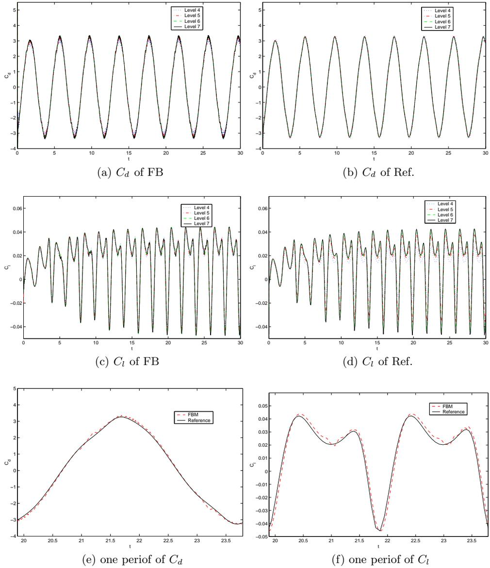
**Fig. 5.** The comparison of  $C_d$  and  $C_l$  between fictitious boundary (FB) and reference (Ref.)
