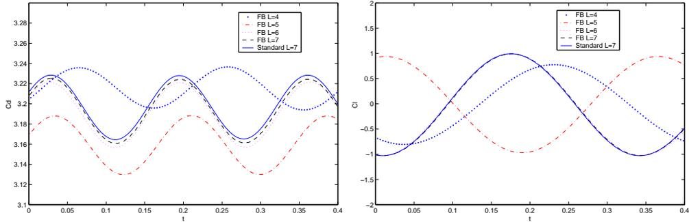
**Fig. 2.** Periodical results of  $C_d$  and  $C_l$  for  $Re = 100$
