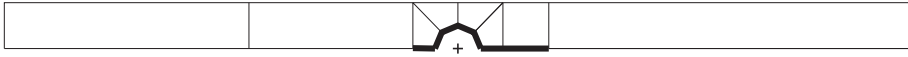
Fig. 4. The coarse mesh for planar flow with a priori local refinement locations.
