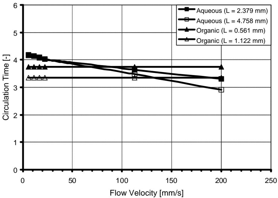
Figure 6: Circulation time inside the liquid slug with respect to the average flow velocity.
