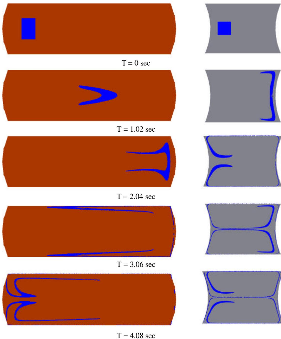
Figure 7: Internal circulations by particle tracing in aqueous and organic slugs respectively.
