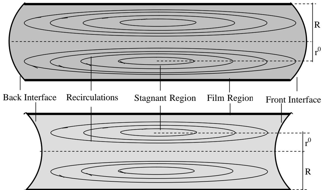
Figure 1b: Schematic representation of internal circulations inside the aqueous and organic slug respectively.
