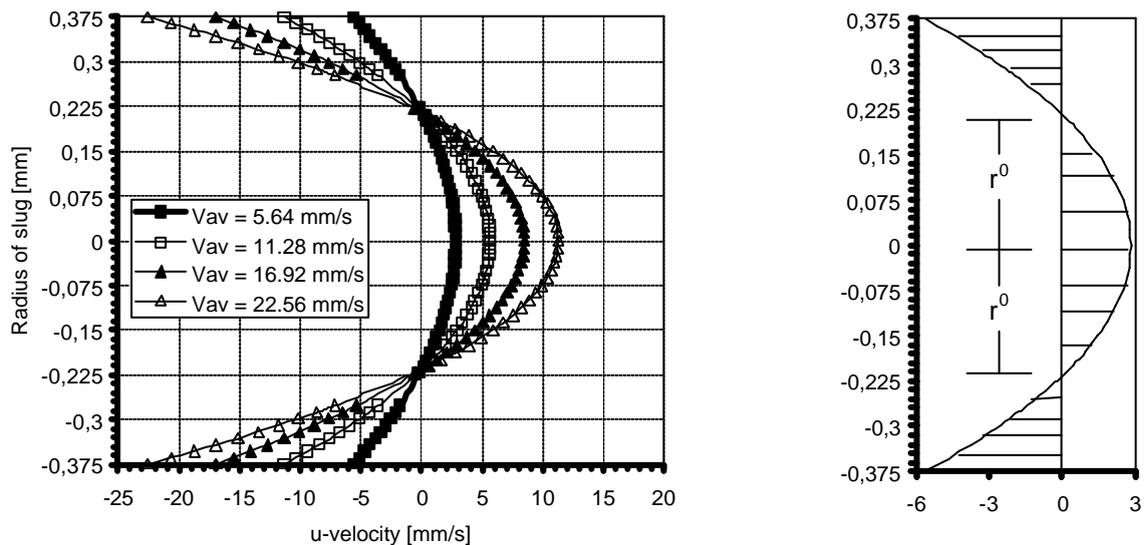
Figure 3b: Parabolic velocity profile inside the slug.
