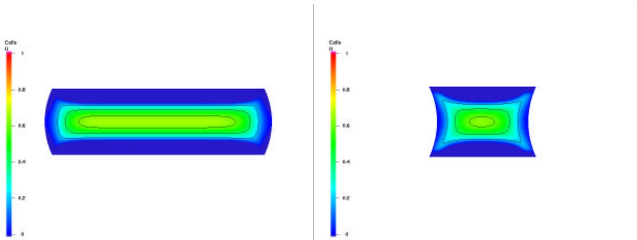
Figure 3a: Contours of velocity in x-direction ( $u$ ) of aqueous and organic slug respectively
