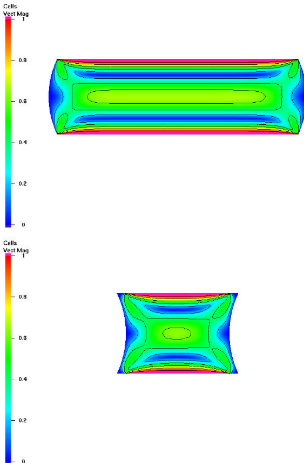
Figure 4. Internal circulations inside the aqueous and organic slug respectively
