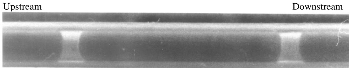
Figure 1a: Liquid-liquid slug flow in a capillary millireactor showing stained aqueous phase and colourless organic phase (Dummann et al., 2003)
