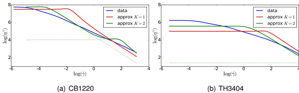
Figure 2: shear viscosities at  $T = 140^\circ\text{C}$
