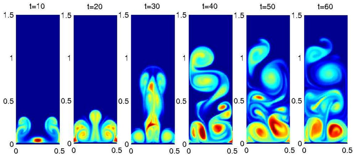
Figure 3. UABC: Na<sub>2</sub>CO<sub>3</sub>,  $w_G = 2 \text{ cm/s}$ ,  $c_{\text{NaOH}}^0 = 1 \text{ mol/l}$ .
