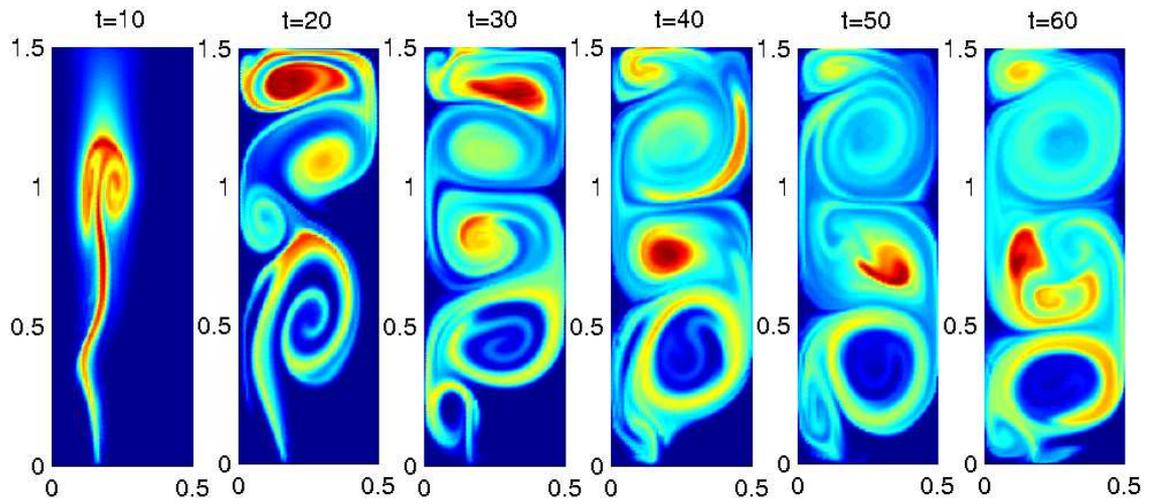
Figure 1. LABC: CO<sub>2</sub>,  $w_G = 0.18 \text{ mm/s}$ , physical absorption.
