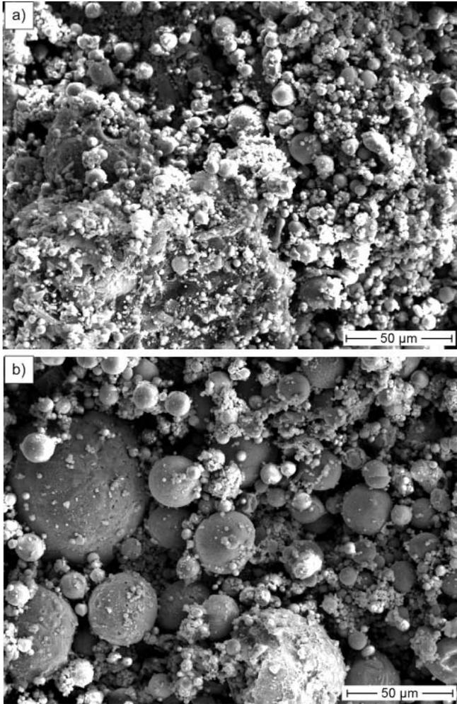
Fig. 4: Variation of particle size along the spray jet of a) Fe- and b) Ni-based particles
