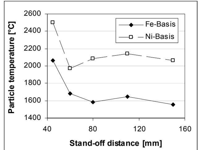
Fig. 5: Variation of particle temperature along the spray jet
