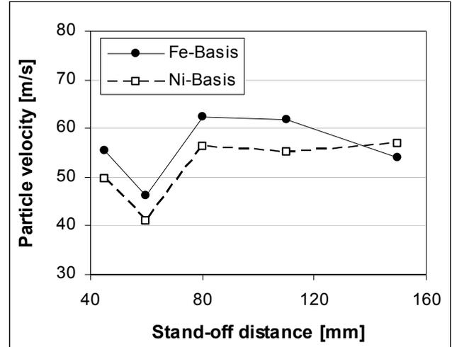
Fig. 2: Variation of particle velocity along the spray jet
