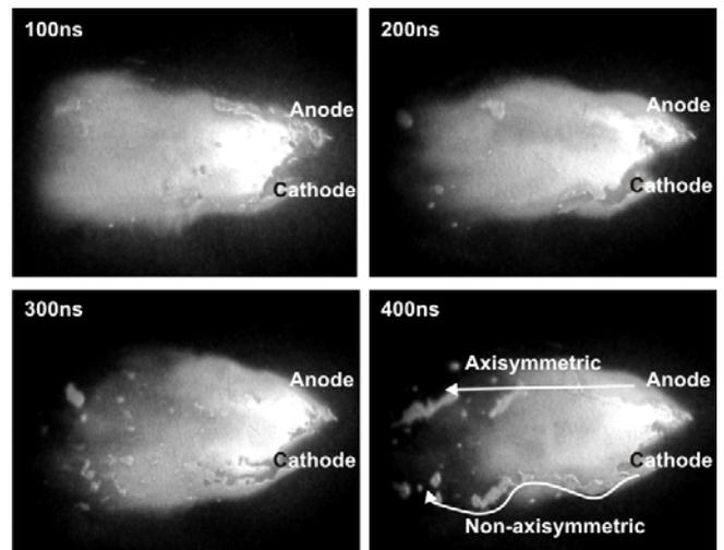
Fig. 3: High speed camera images of Fe-based wires at different sequences
