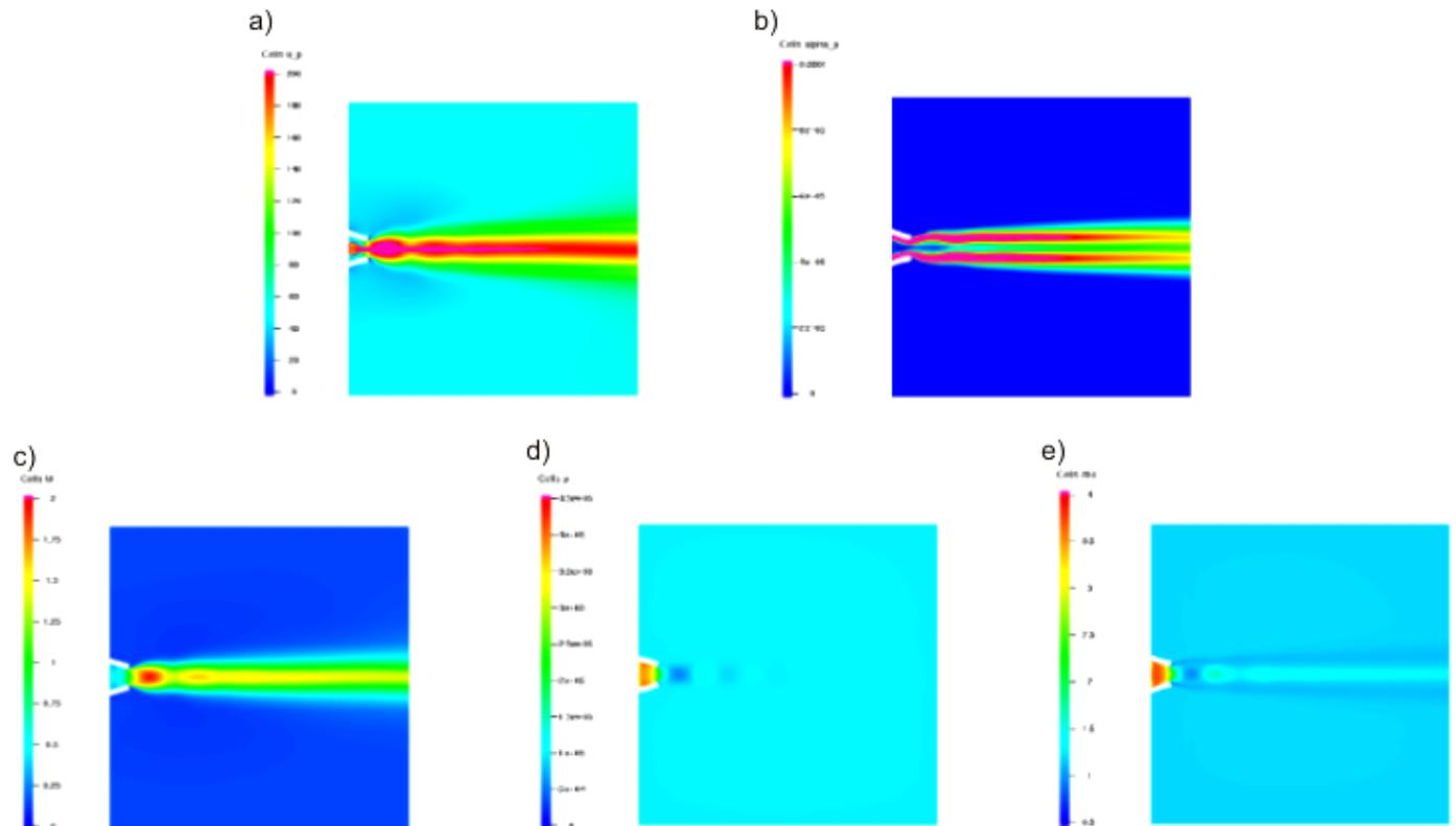
**Fig. 1:** Numerical results of a) particle velocity in m/s; b) volume fraction of particles in %; c) Mach number of the gas; d) gas pressure in Pa and e) gas density  $\text{kg/m}^3$
